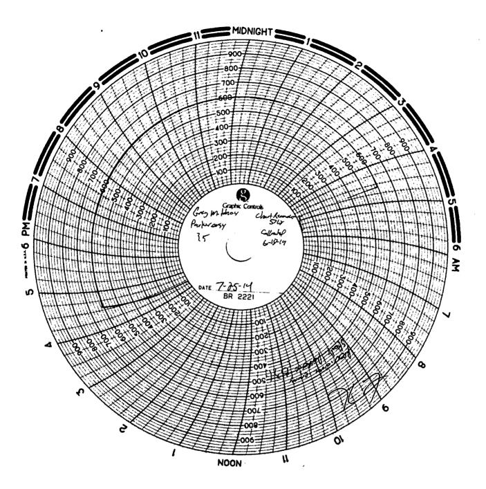
July 25, 2019 Providence Energy Services, Inc dba Kelton Operating Skelly Penrose B Unit #31 API #30-025-10639 Scheduled MIT Test Parker Energy Services Truck #35 - Greg Meter #5762 Calibrated June 18, 2019
