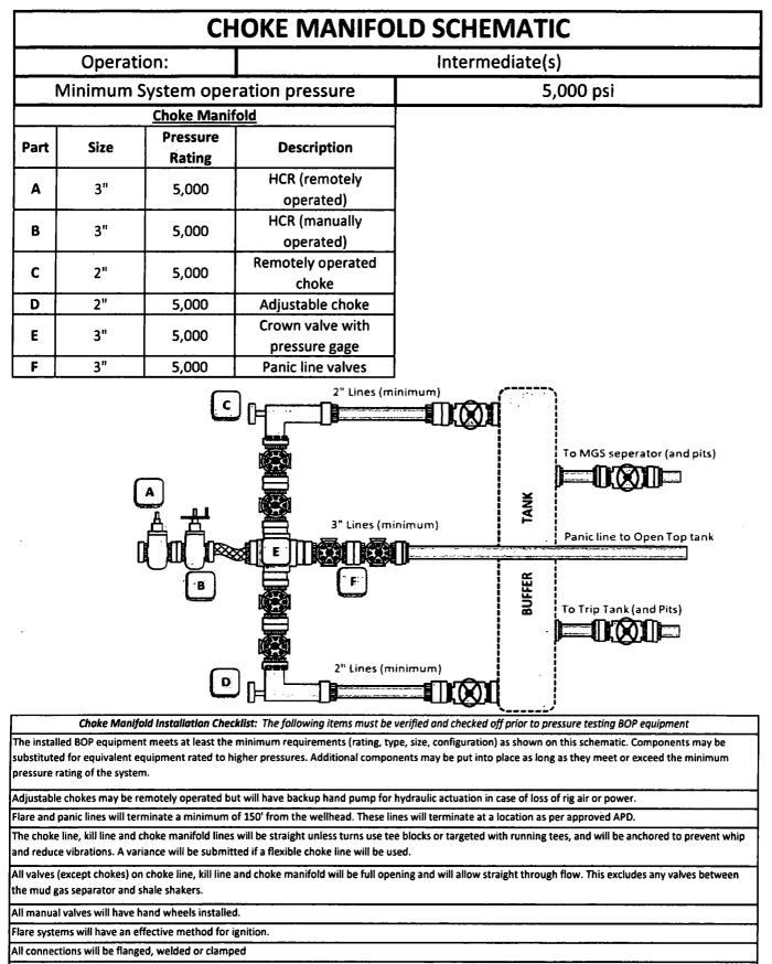
If buffer tank is used, a valve will be used on all lines at any entry or exit point to or from the buffer tank.
