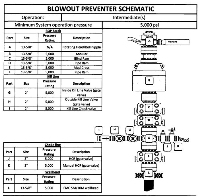
BOP Installation Checklist: The following items must be verified and checked off prior to pressure testing BOP equipment
