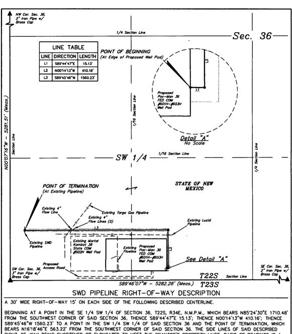
RIGHT-OF-WAY BEING SHORTENED OR ELONGATED TO MEET THE GRANTOR'S PROPERTY LINES. BASIS OF BEARINGS IS A TRANSVERSE MERCATOR PROJECTION WITH A CENTRAL MERIDIAN OF W103'53'00". CONTAINS 1.367 ACRES MORE OR LESS.
