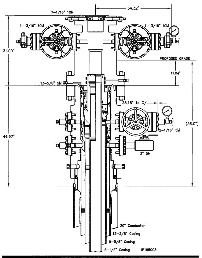
IP1042 Rev. 0 Page 2 Caza Petroleum 20" x 13-3/8" x 9-5/8" x 5-1/2" 5/10M MBU-3T-CFL-R-DBLO Wellhead System With CTH-DBLHPS Tubing Head
