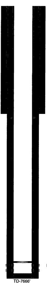
11" hole @ 3150' 8-5/8" csg @ 3150' w/ 2000sx-TOC-Surf-Circ
