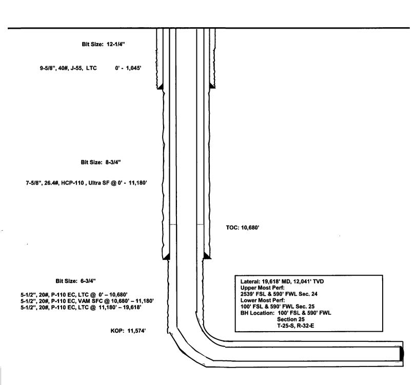
2167' FSL 590' FWL Section 24 T-25-S, R-32-E Proposed Wellbore Design B KB: 3,465' GL: 3,440'
