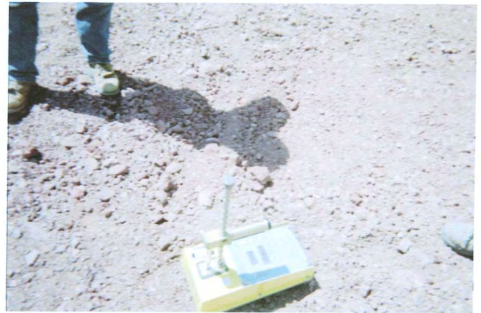
Clay compaction test being performed
