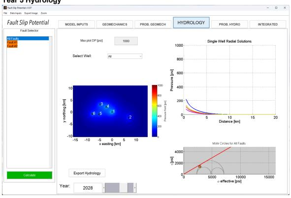
Year 5 Probabilistic Hydrology (note no crossover between blue delta-press. & green fault slip press.)
