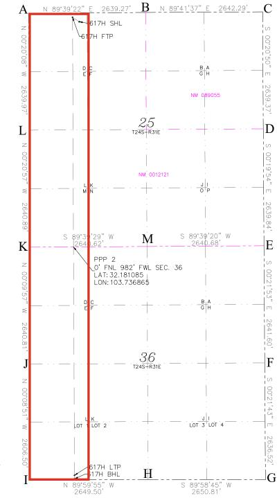
$\begin{array}{l} A= N:435400.07 \quad E:724859.41 \\ B= N:435415.91 \quad E:727498.63 \\ C= N:435430.04 \quad E:730140.88 \\ D= N:432790.73 \quad E:730156.88 \\ E= N:430150.93 \quad E:730172.17 \\ F= N:427509.39 \quad E:730188.98 \\ G= N:424872.92 \quad E:730205.63 \\ H= N:424871.96 \quad E:727554.82 \\ I= N:424872.01 \quad E:724905.32 \\ J= N:427478.51 \quad E:724898.61 \\ K= N:430119.30 \quad E:72489.97 \\ L= N:432760.15 \quad E:724874.87 \\ M= N:430135.06 \quad E:727531.54 \\ \end{array}$
