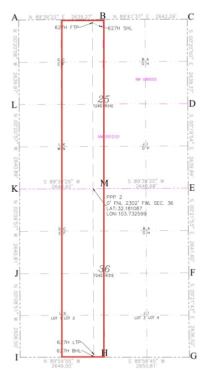
A=N:435400.07 E:724859.41 B=N:435415.91 E:727498.63 C=N:435430.04 E:730140.88 B=N:432790.73 E:730172.17 F=N:427509.39 E:730178.17 F=N:427509.39 E:730188.98 G=N:424872.92 E:730205.63 H=N:424871.96 E:727554.82 I=N:424872.01 E:724905.32 J=N:427478.51 E:724898.61 K=N:430119.30 E:724890.97 M=N:430135.06 E:727531.54
