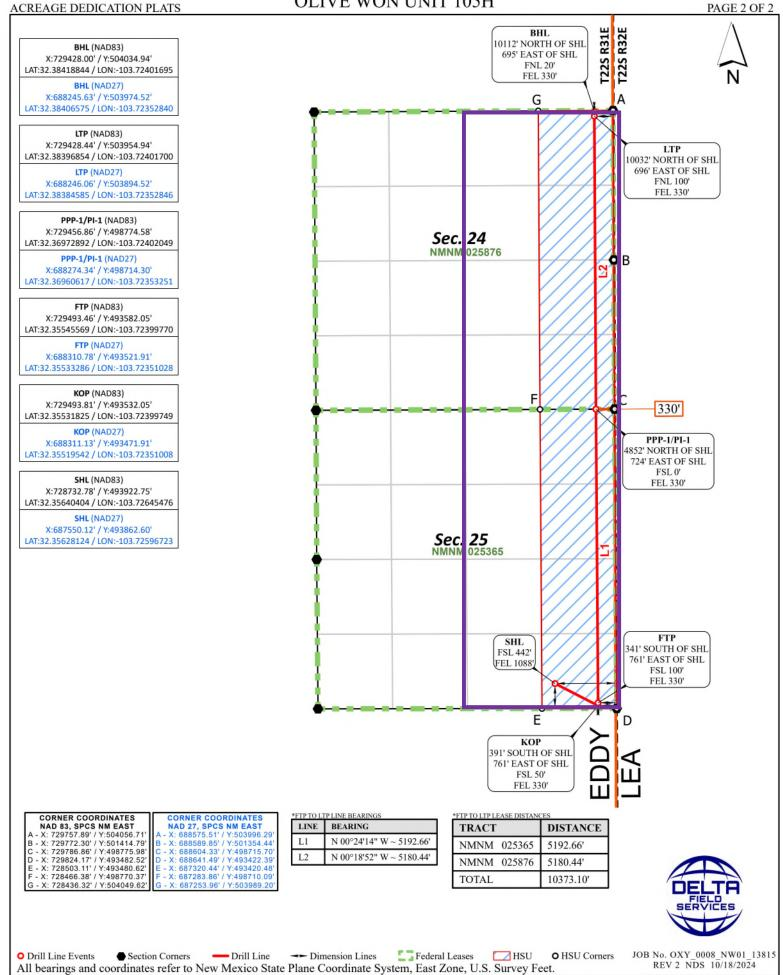
Distances/areas relative to NAD 83 grid measurements. Combined Scale Factor: 0.99978405 and a Convergence Angle: 0.31759200°
