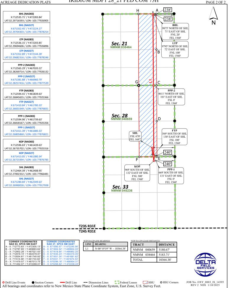
Distances/areas relative to NAD 83 grid measurements. Combined Scale Factor: 0.99977581 and a Convergence Angle: 0.27195833°
