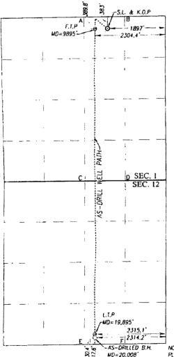
SCALE: 1"=2000 GEODETIC COORDINATES GEODETIC COORDINATES NAD 27 NAE NAD 83 NAE SURFACE LOCATION & SURFACE LOCATION & KICK OFF POINT KICK OF POINT Y=393041.7 N Y=.393099.2 N X=719226.7 E X=7604133 E LAT. = 32,078610 N LAT. = 32,078735° N LONG. = 103.625542 W LONG. = 103.626013" W FIRST TAKE POINT FIRST TAKE POINT NAD 27 NIME NAD 83 NME Y=393029.7 N Y=393087.2 N X=718819.0 E x=760005.6 E LAT. = 32.078585° N LAT.=32.078709 N LONG. = 103.626858" W LONG. = 103.627329° W CORNER COORDINATES TABLE
