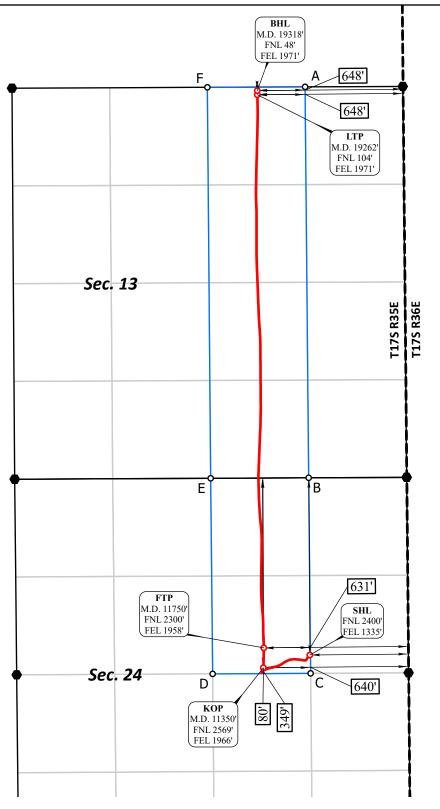
CORNER COORDINATES NAD 83, SPCS NM EAST A - X: 825924.42' / Y:671324.32' B - X: 825972.86' / Y:666030.12' - X: 825999.32' / Y:663382.16' - X: 824672.87' / Y:663374.87' - X: 824646.03' / Y:666023.82' - X: 824601.31' / Y:671318.24'
