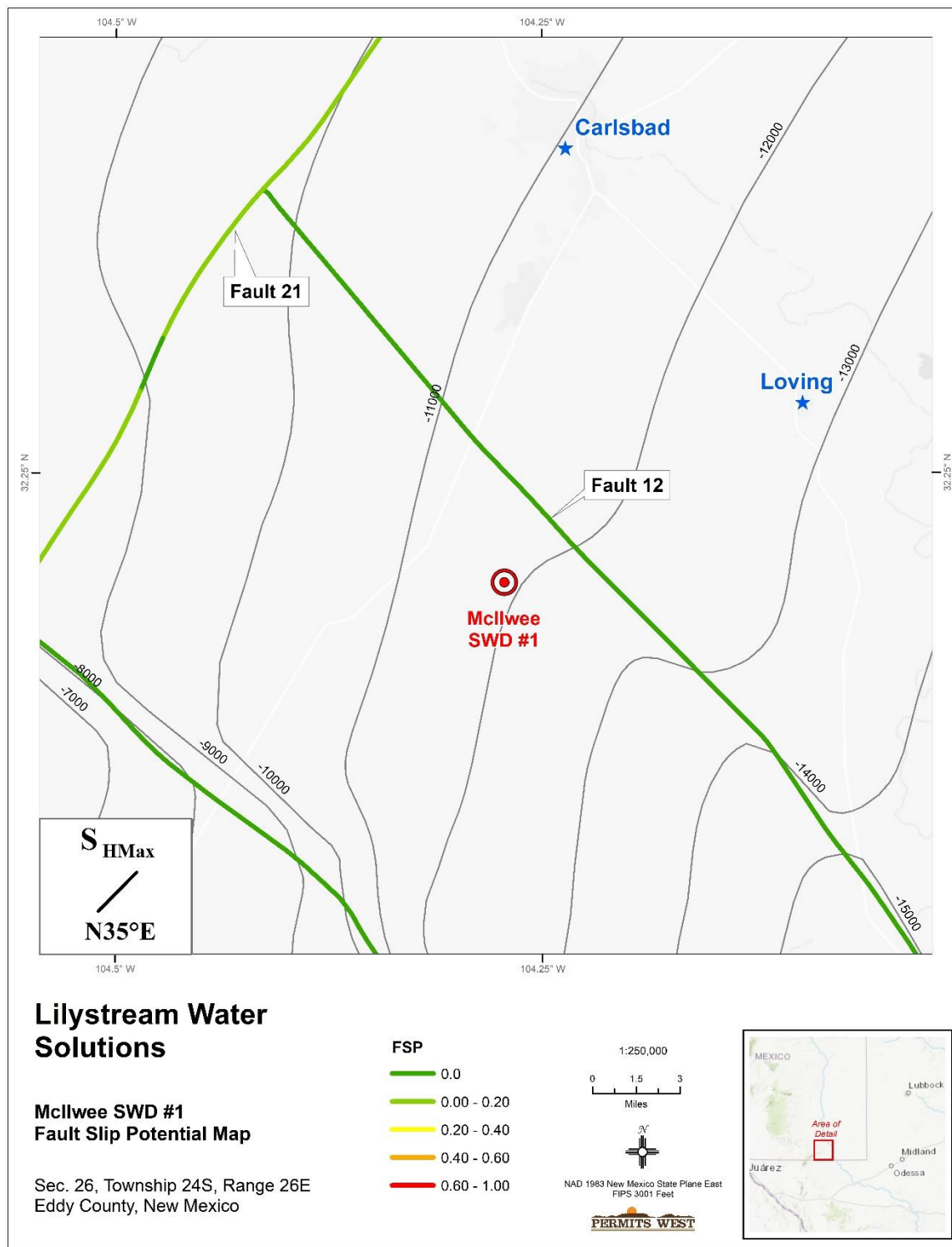
Figure 2. Precambrian fault map of the McIlwee SWD #1 area as mapped by Horne et al. (2021). Faults are colored based on probability of fault slip as modeled using Fault Slip Potential software (Walsh and Zoback, 2016). Labeled values represent the calculated fault slip potential using the parameters indicated in Table 2. Contours show the top of the Precambrian basement in feet below sea level.
