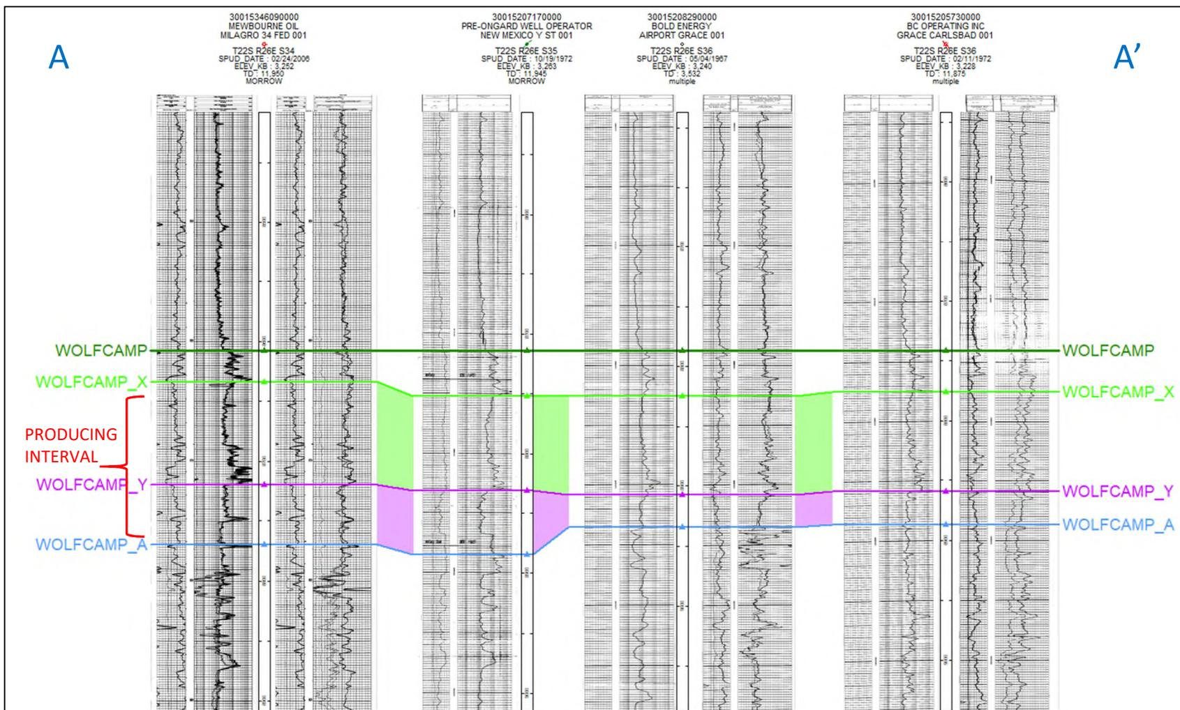
Line of section showing the continuity, thickness and lack of faulting in the Wolfcamp X/Y target zone.
