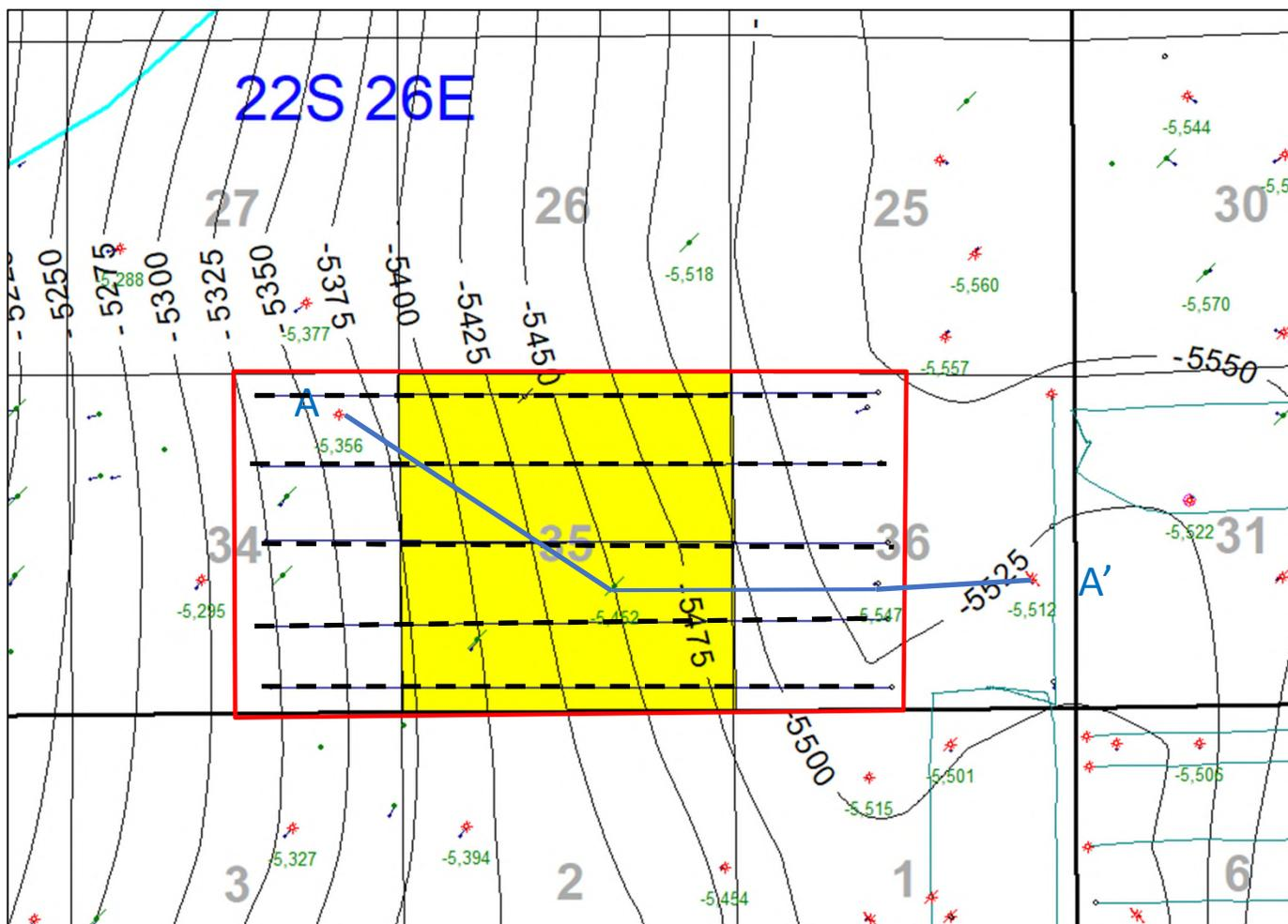
Contours are subsea Top Wolfcamp. Control wells have green dots and green subsea values. Map shows uniformity and continuity of Wolfcamp section.
