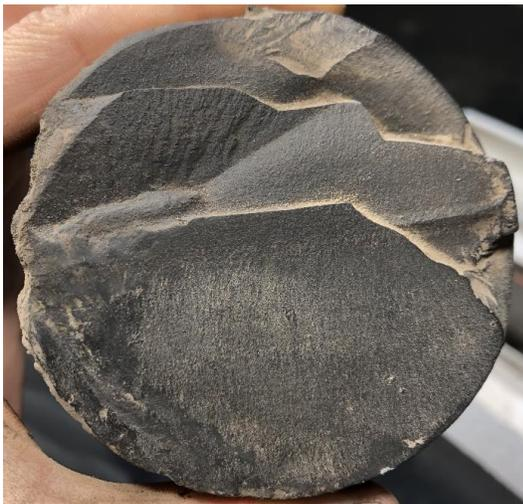
Fig 61—(a) fracture face showing sand patches (b) close-up of patch, field of view ~1 cm. (c) cleaned face showing steps and twist hackles.
