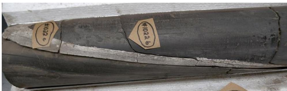
Fig 58—(a) Discontinuous, bed-parallel fractures with blocky fill. Core 4, (b) Thick (1 cm) beef in Core 9. Labels are for core-handling breaks.
