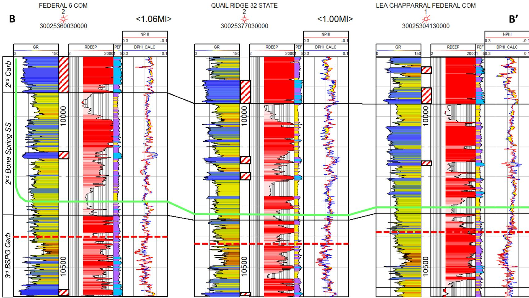
PR's additional 3<sup>rd</sup> Carb target lies ~135' below L. 2<sup>nd</sup> Sand target. No significant frac baffle separates the two reservoirs.
