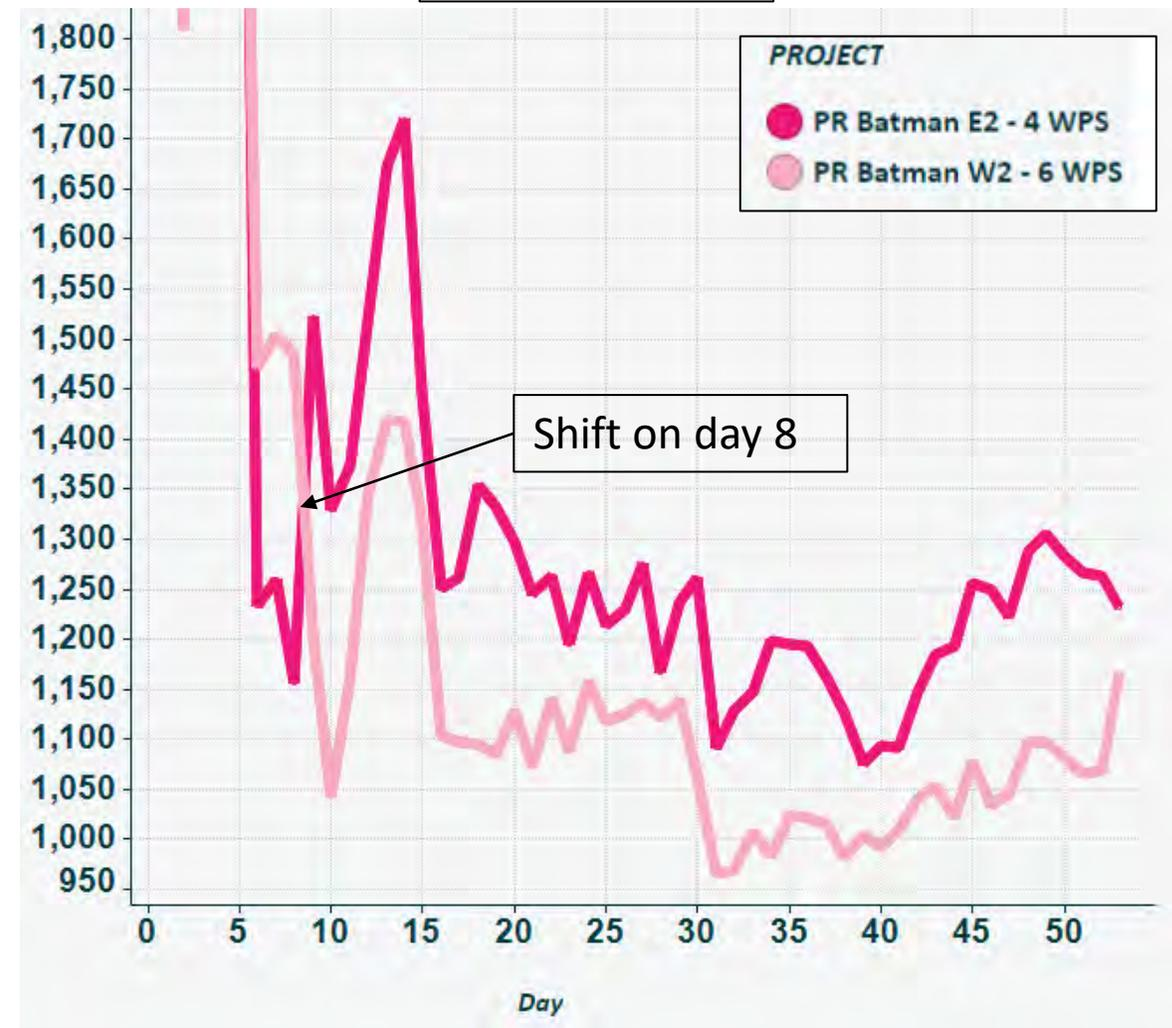
Shift in oil allocation on day 8, long-term trend or driven by a hung separator dump or carryover?
