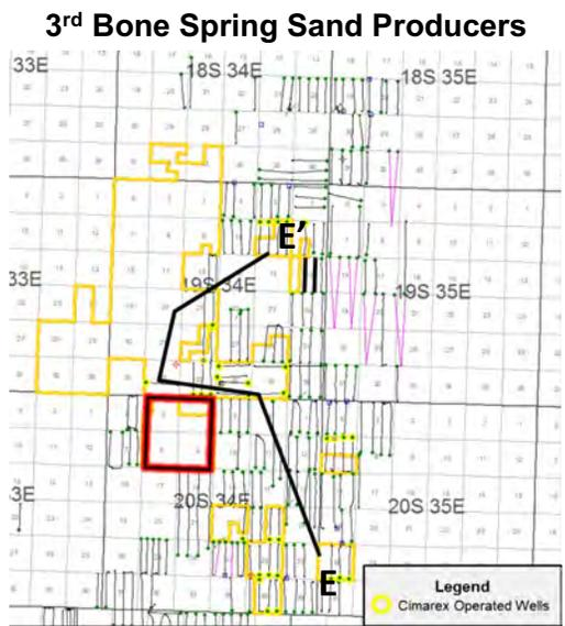
Basal 3<sup>rd</sup> Sand is primary target across the area (green line). Frac baffles are not located between the 3<sup>rd</sup> Sand target and Upper Wolfcamp across these developments. Example of a frac baffle that would most likely prevent communication between formations is within the 3<sup>rd</sup> Carbonate in the Chief 30 State 3H log.
