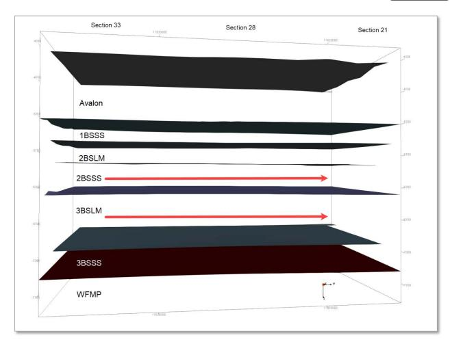
**WPX Exhibit B-5** Three-dimensional structural cross section with approximate well trajectory shown by red arrows.
