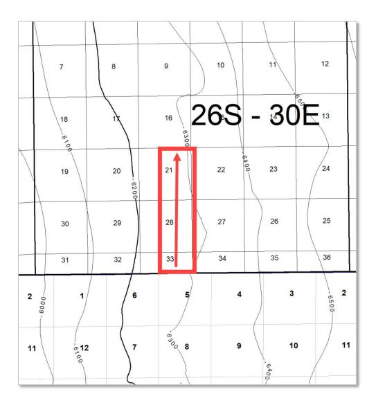
**WPX Exhibit B-1** is a structure map showing the depth (subsea) to the top of the  $3^{rd}$  Bone Spring Limestone, a key marker between the two landing zones of the proposed wells. Red arrow indicates well direction. Contour inverval = 100'
