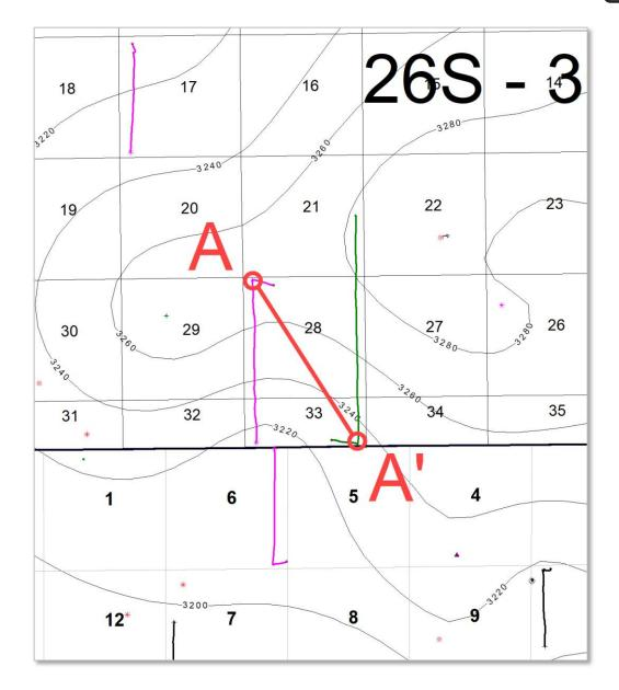
**WPX Exhibit B-3** Gross isochore from the top of Bone Spring to top of Wolfcamp with a 20' contour interval. Map demonstrates continuity and consistent thickness of formation.
