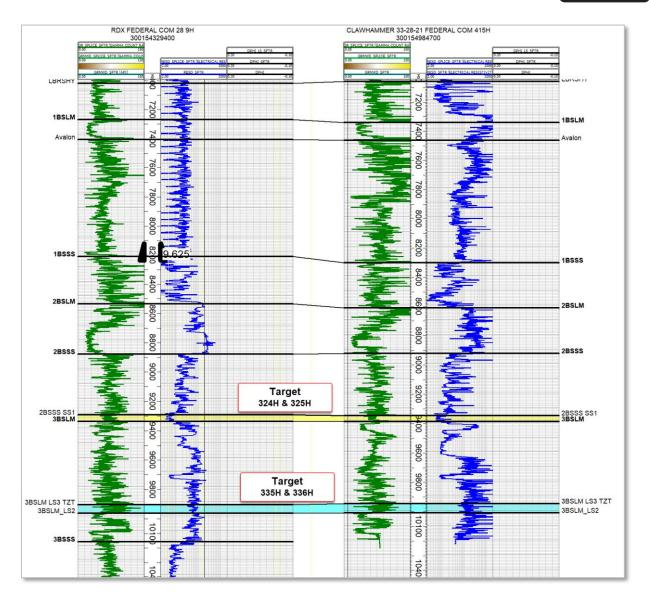
**WPX Exhibit B-2** Cross-section A to A'. Stratigraphic cross-section flattened on top of the 3<sup>rd</sup> Bone Spring Limestone. Target intervals indicated with well numbers.
