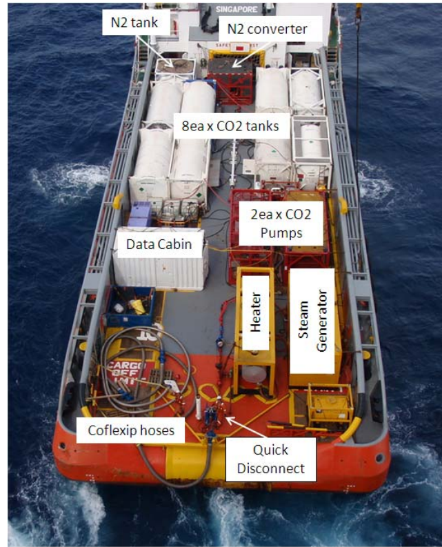
Fig.5 – Layout of the CO2 equipment on the work boat
