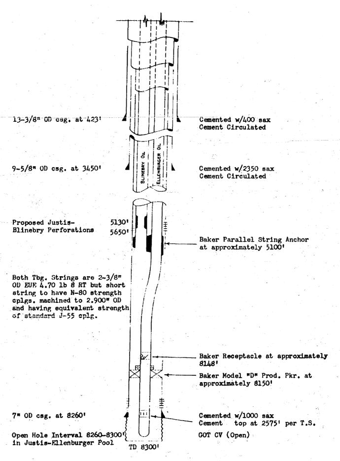
PROPOSED MECHANICAL INSTALLATION OIL-OIL DUAL COMPLETION
