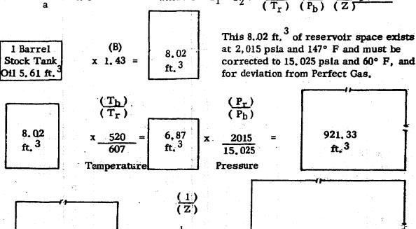
(1) This is the volume of gas which will occupy the same reservoir space as one barrel of stock tank oil and its solution gas.
