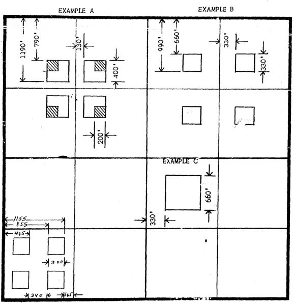
EXAMPLE A - Shows Standard Gas Well location in San Juan, Rio Arriba and Sandoval Counties. 200' crosshatched square shows portion of 400' square which is a standard location for oil or gas wells. These locations may be used in any quarter section.
