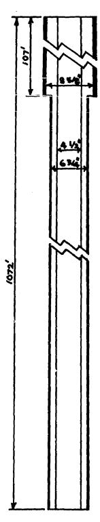
Surface pipe cemented w/50 Sax of regular cement w/2% c.c.
