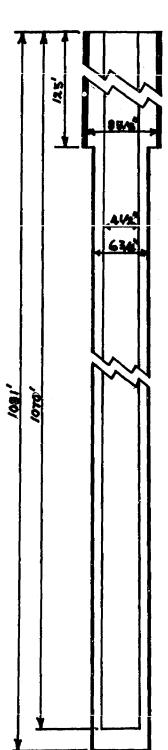
Surface pipe cemented w/50 sax of regular cement w/2%c.c.
