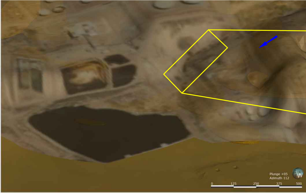
LOCAL SURFACE TOPOGRAPHY SHOWING SWALE IN THE HYDROCARBON SEEP AREA EAST VIEW, X5 VERTICAL EXAGGERATION
