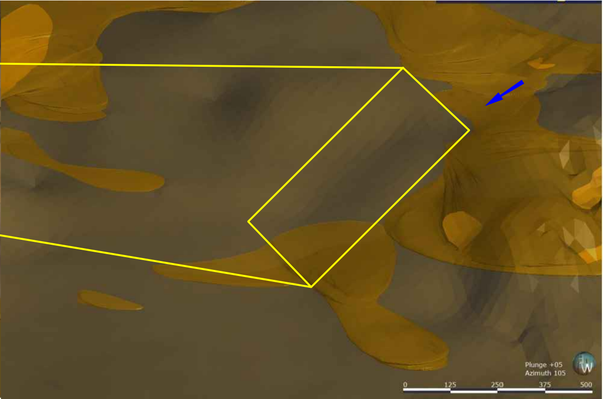
GEOLOGICAL MODEL SHOWING SWALE IN SHALLOW ALLUVIAL DEPOSITS (FINE - DARK, COARSE - LIGHT) IN THE HYDROCARBON SEEP AREA EAST VIEW, X5 VERTICAL EXAGGERATION
