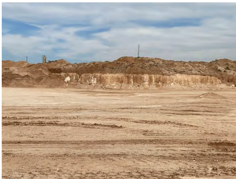
Image 3 – Caliche mine 2.7 miles south of the Longhorn Facility which exposes the 8 to 10-foot-thick layer of caliche.
