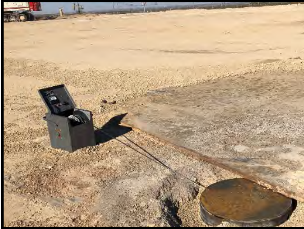
Image 10 - We did not encounter groundwater to a depth of 55 feet at a future COG Operating well.
