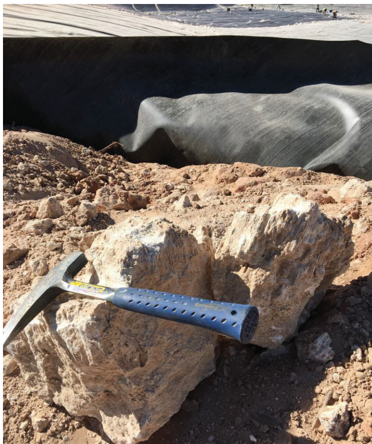
Figure 2: Chemically weathered gypsum near the anchor trench of the northern excavation; Liner installation in top-background.
