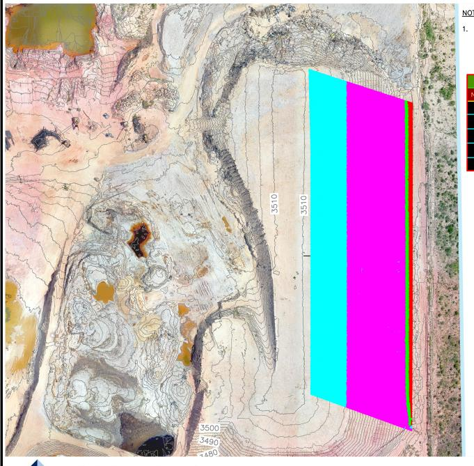
NEGATIVE ELEVATIONS INDICATE ADDITIONAL FILL NEEDED TO REACH FINAL GRADE, POSITIVE ELEVATIONS INDICATE FILL ABOVE GRADE.
