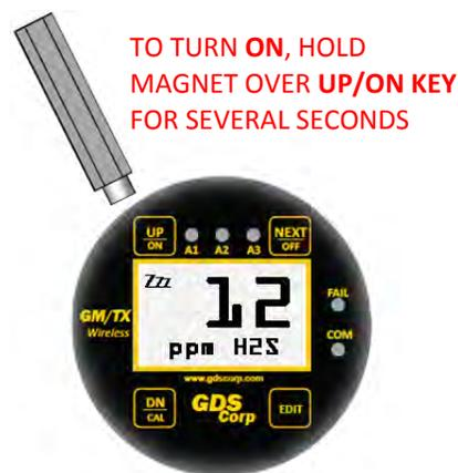
Figure 4-1: GASMAX TX Display
