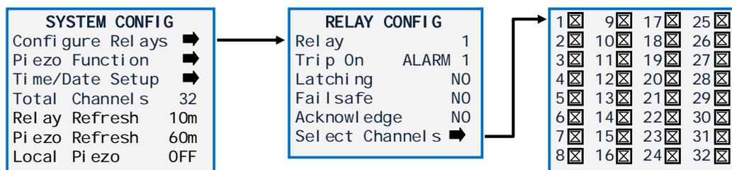
**Figure 10-3: System Config – Relay Config Menu**
