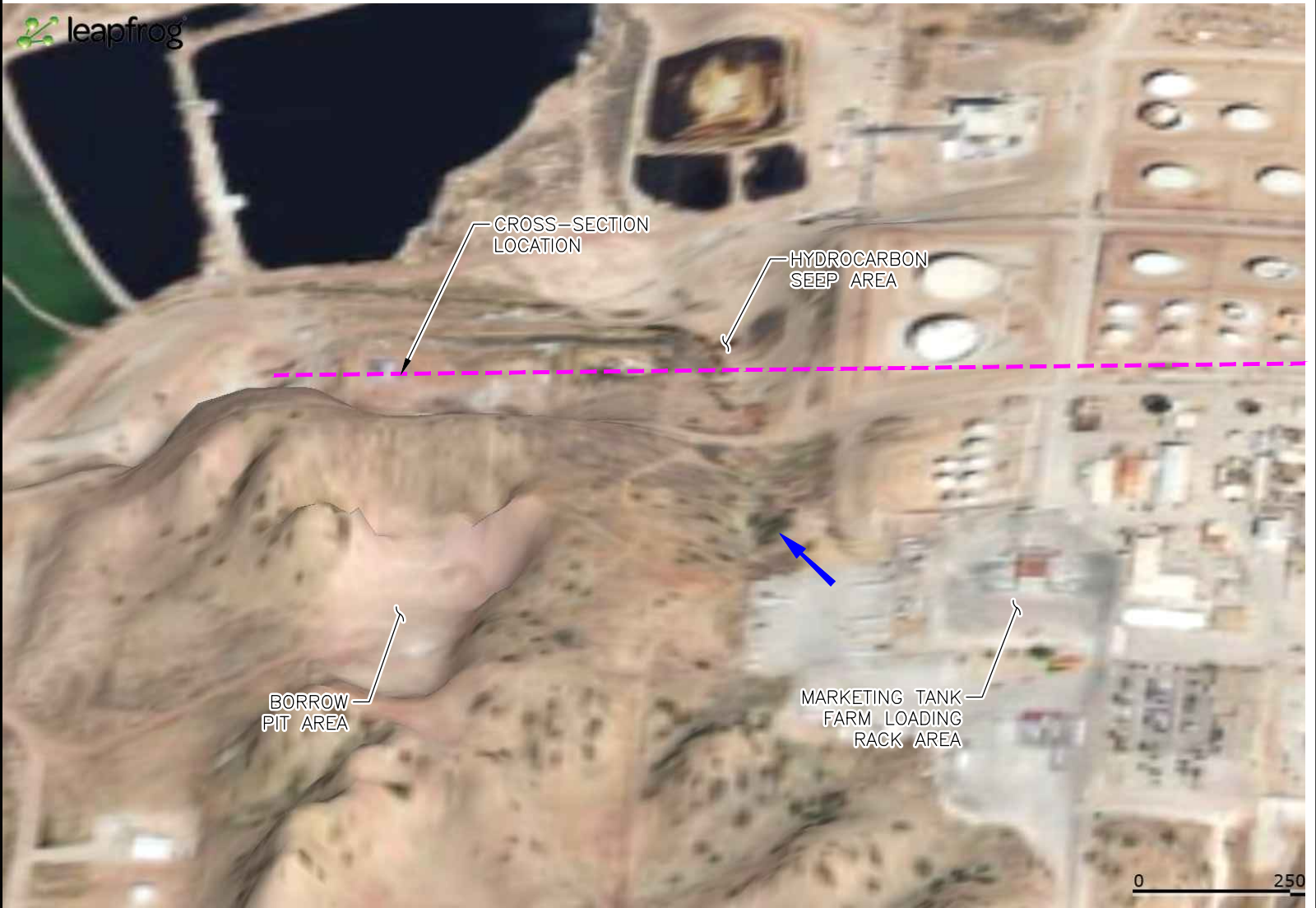
LOCAL SURFACE TOPOGRAPHY SHOWING SWALE IN THE HYDROCARBON SEEP AREA NORTH VIEW, X5 VERTICAL EXAGGERATION
