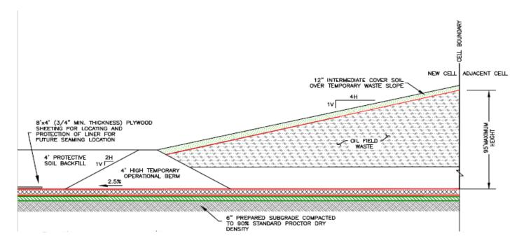
While this does not prevent the shifting of waste, it does give the site personnel and area of reference of where waste can be placed in the cell, thereby protecting the tie in point from heavy equipment working in the cell
