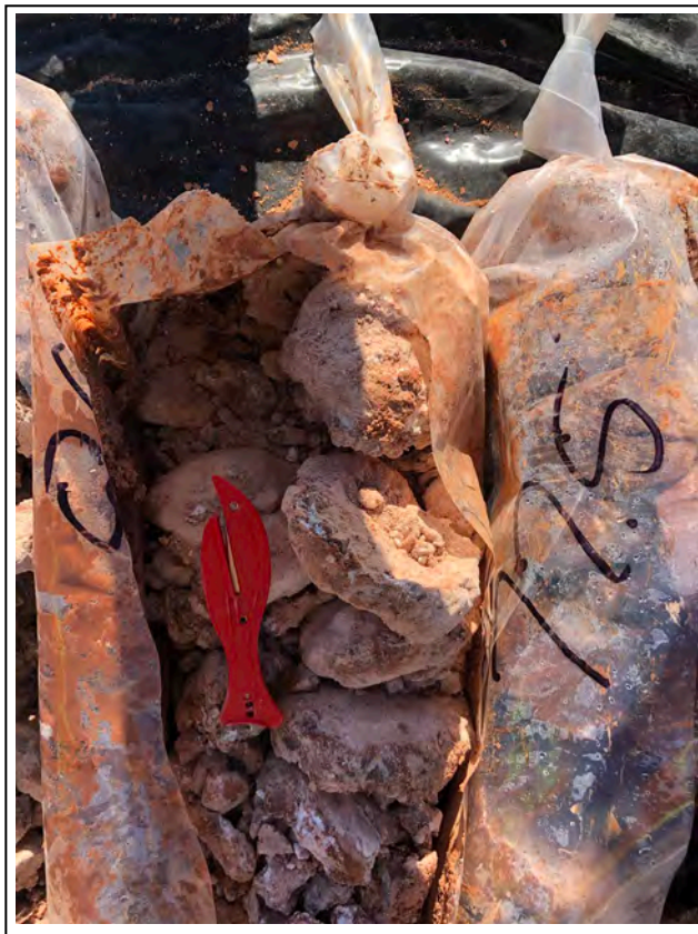
7. Core sample at 80 feet bgs
