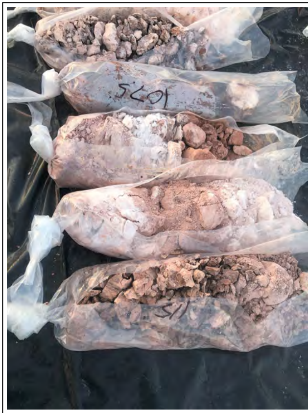
11. Core samples from 105 to 115 feet bgs
