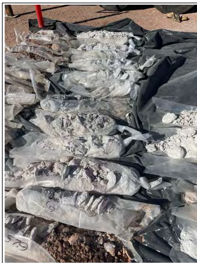
6. Core samples from 62.5 to 95 feet bgs
