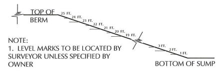
2. MARKS TO BE MADE BY AN EXTRUSION WELDER USING BLACK FILAMENT (OR WHITE FILAMENT ON BLACK LINER).
