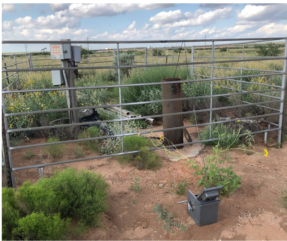
Figure 9 – Measuring depth to groundwater in south well (MISC-161) in 2021
