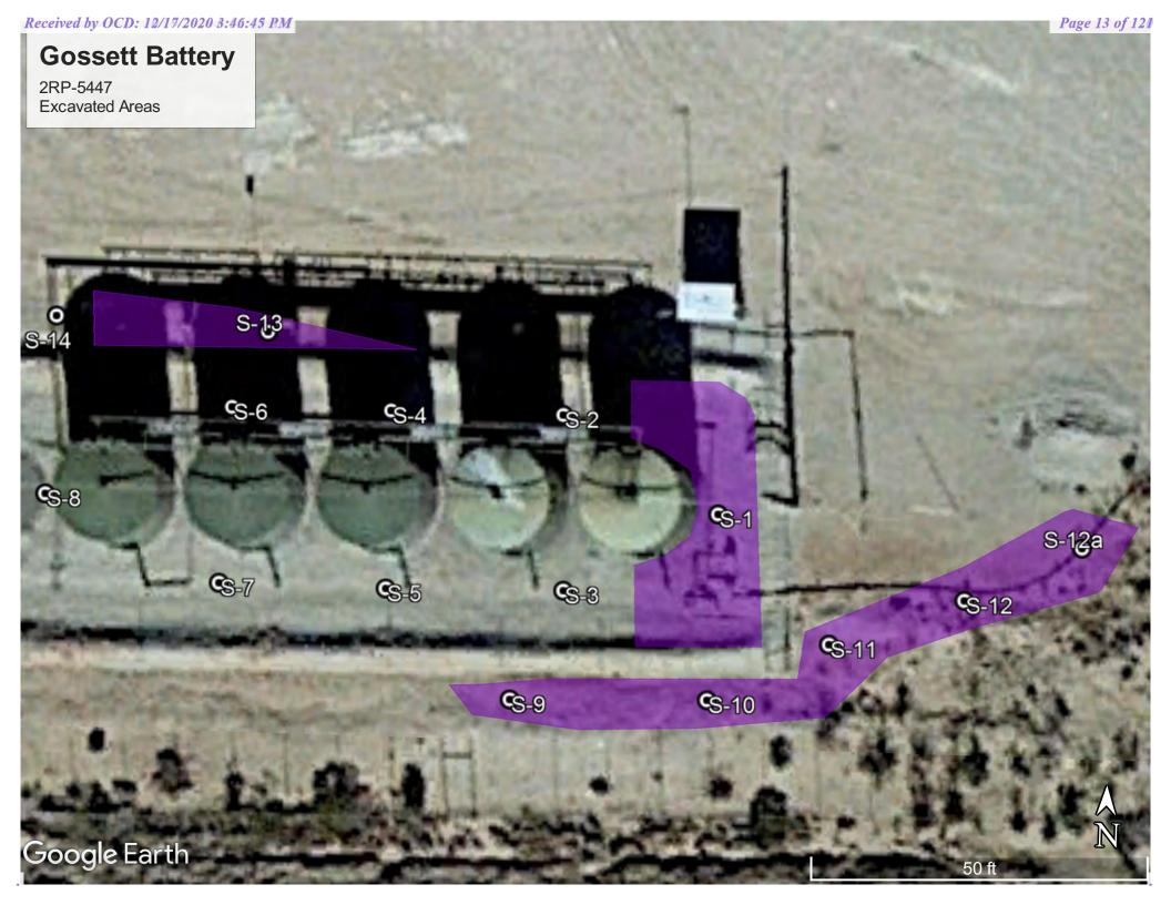
2RP-5447 Gossett Battery Spill Soil Sample Results
