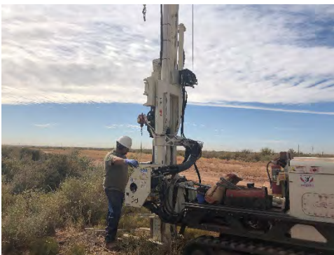
9. View of Geoprobe advancing a soil boring along right of way.
