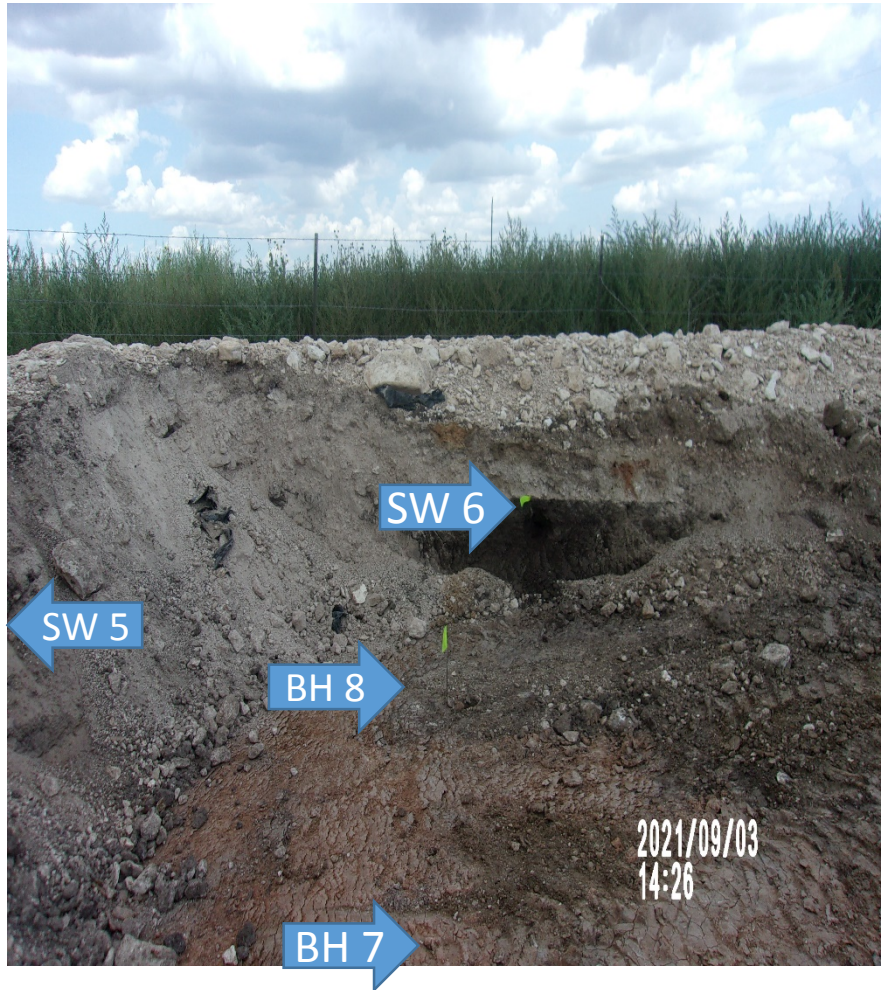
View South – Sample location Bottom Hole 7 (3' EB), Bottom Hole 8 (3' EB), Side Wall 5 and Side Wall 6 (flagged). Blue arrow identifies pin flag.
