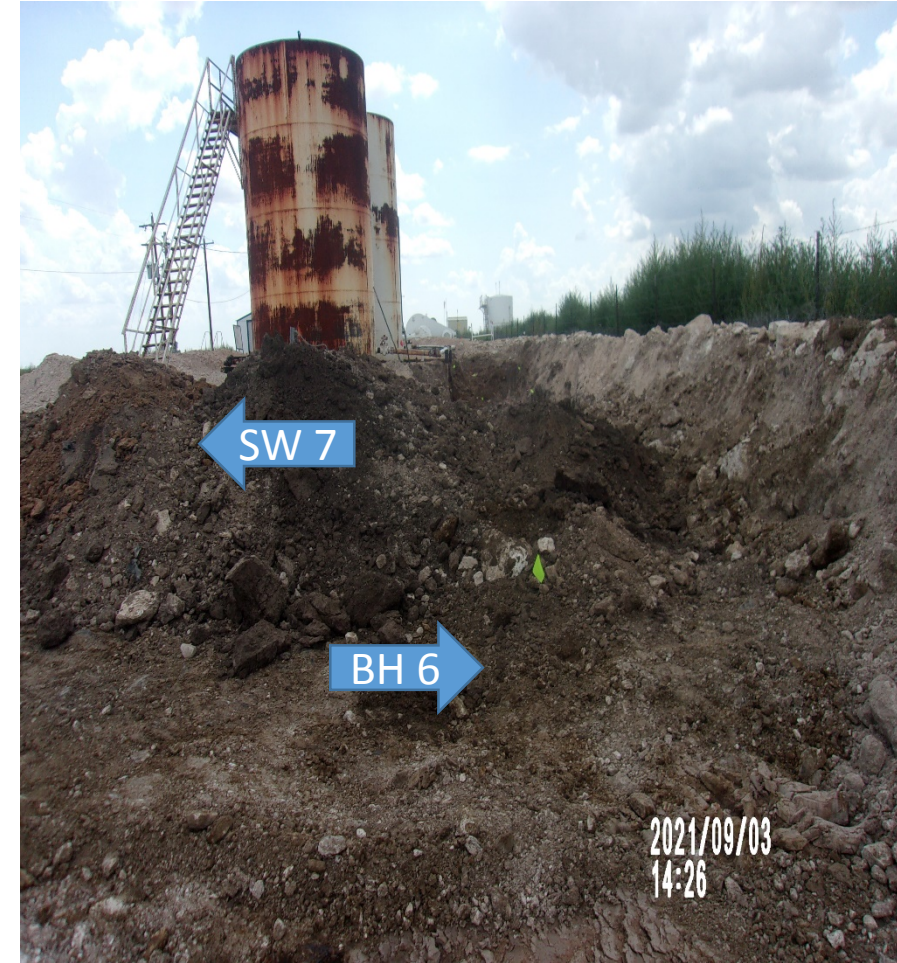
View South – Sample locations Bottom Hole 6 (3' EB) and Side Wall 7 (flagged). Blue arrows identify pin flags.
