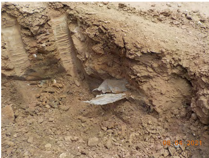
Typical view of plastic liner encountered in test holes located over apparent closed pit.
