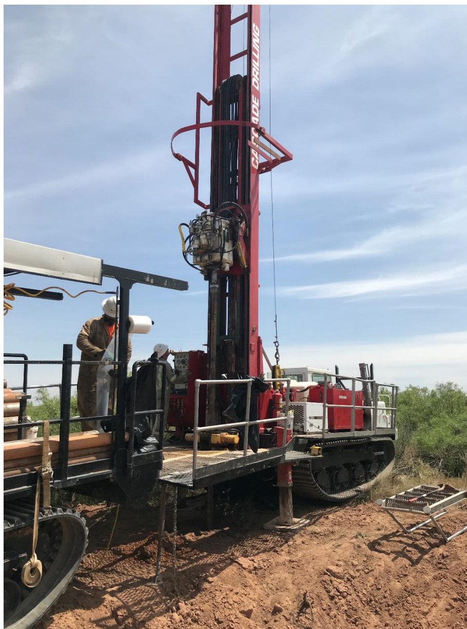
Track-mounted sonic drill rig utilized for the advancement of boreholes
