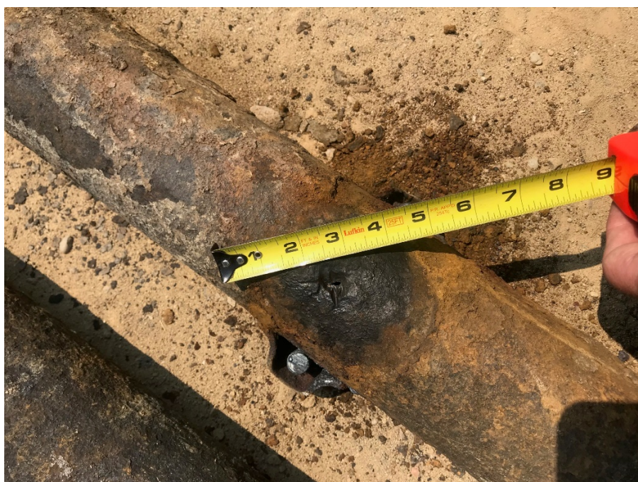
Photo 2: Hole in 4-inch pipe.
