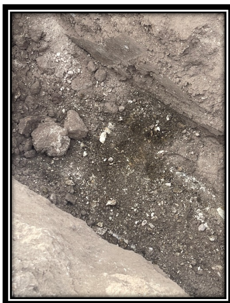
Picture 12: Competent Base With Residual Potassium Permanganate
