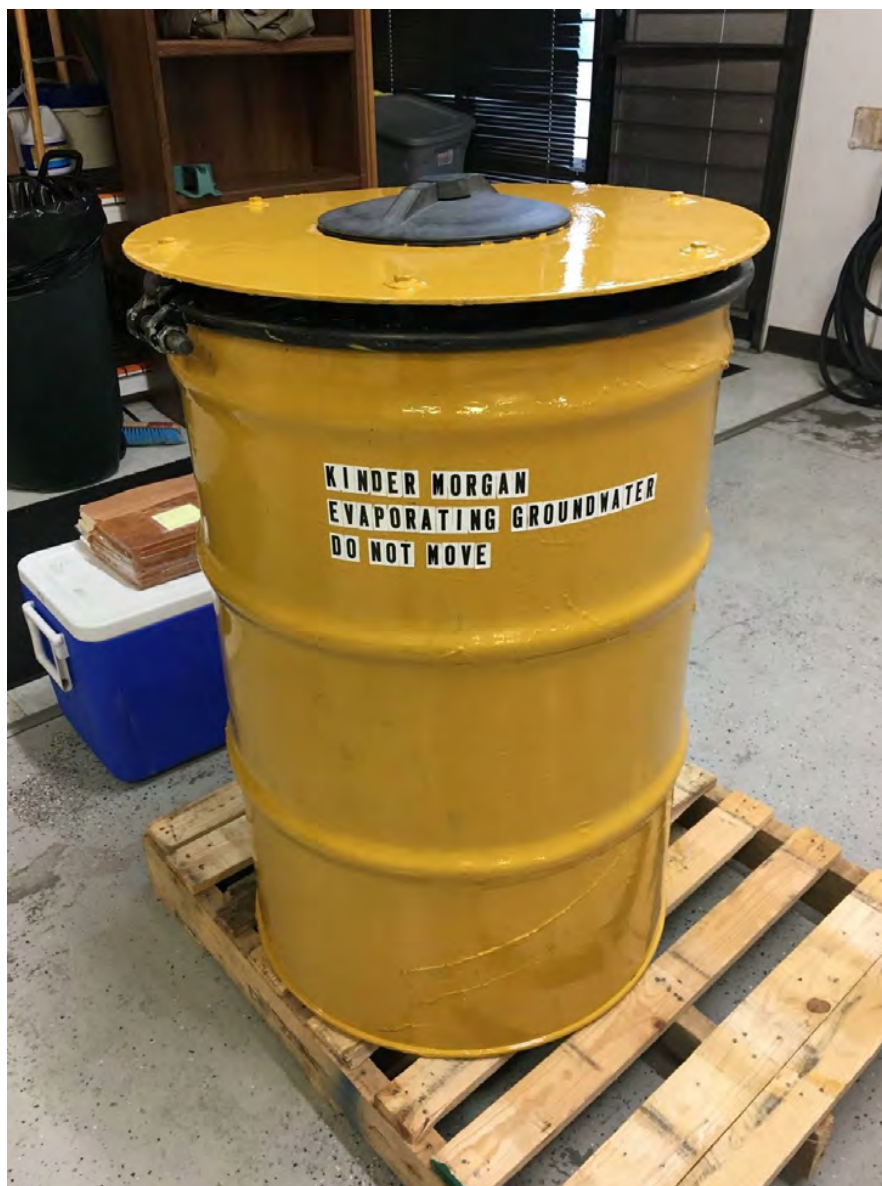
Jal #4 Gas Plant, Jal, New Mexico – Drum with Ventilated Barrel Cover
