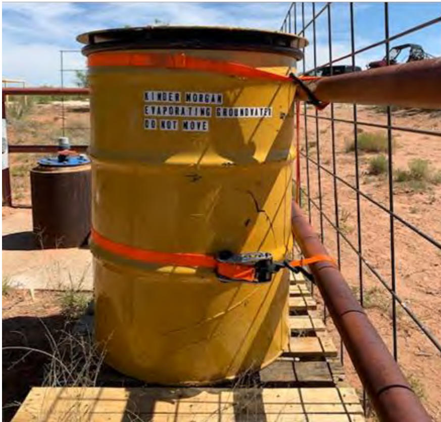
Jal #4 Gas Plant, Jal, New Mexico - Field-Deployed Drum with Ventilated Barrel Cover – Evaporates Groundwater Monitoring IDW Purgewater “24-7”
