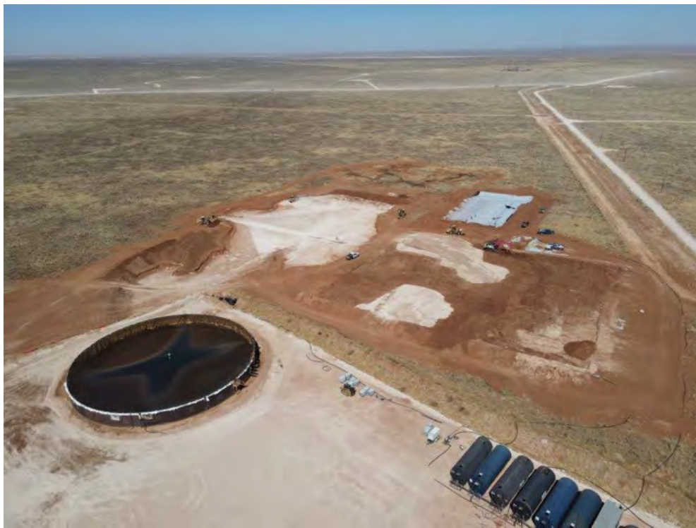
Figure: A drone image shows the lined treatment cell adjacent to the spill area
