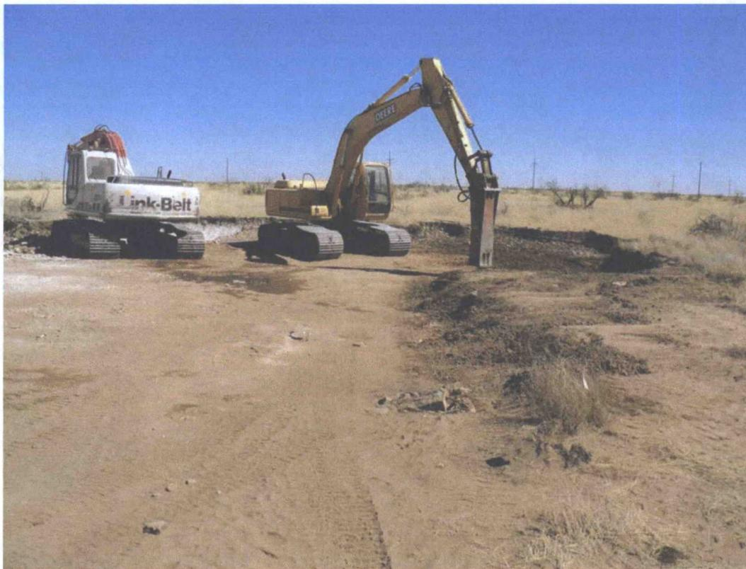
**Photograph No. # 3 – Trackhoes with Rock Bucket (left) and Hammerhoe attachment (right)**
