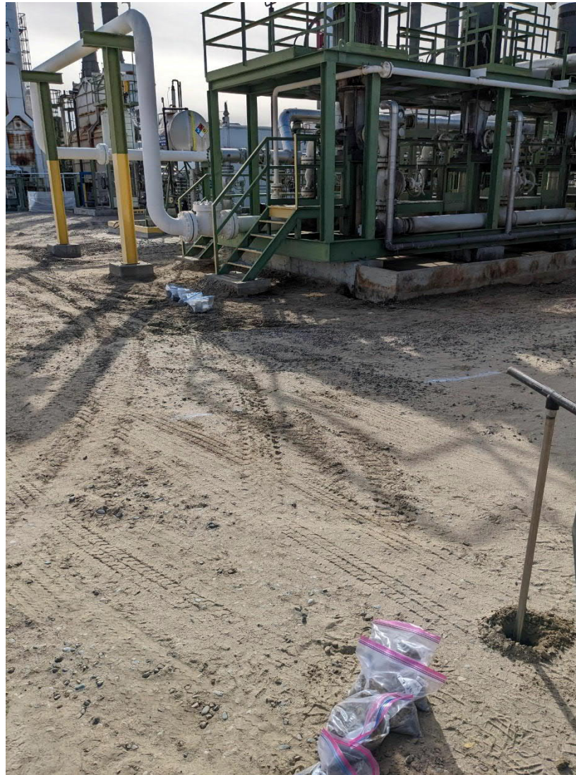
Photo #3 Hand auger delineation outside of excavation extent.
