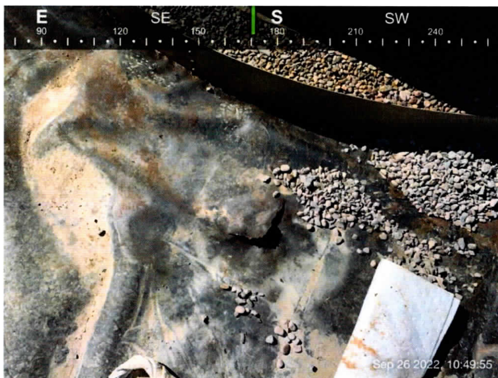
Photo 3: Hole in liner, 9/26/2022.
