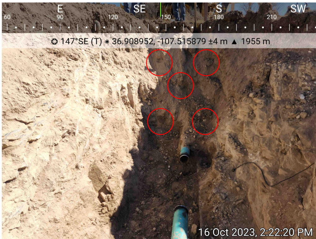
Photo 4: SS03 is a five-point composite sample collected from south sidewall, 10/16/2023.
