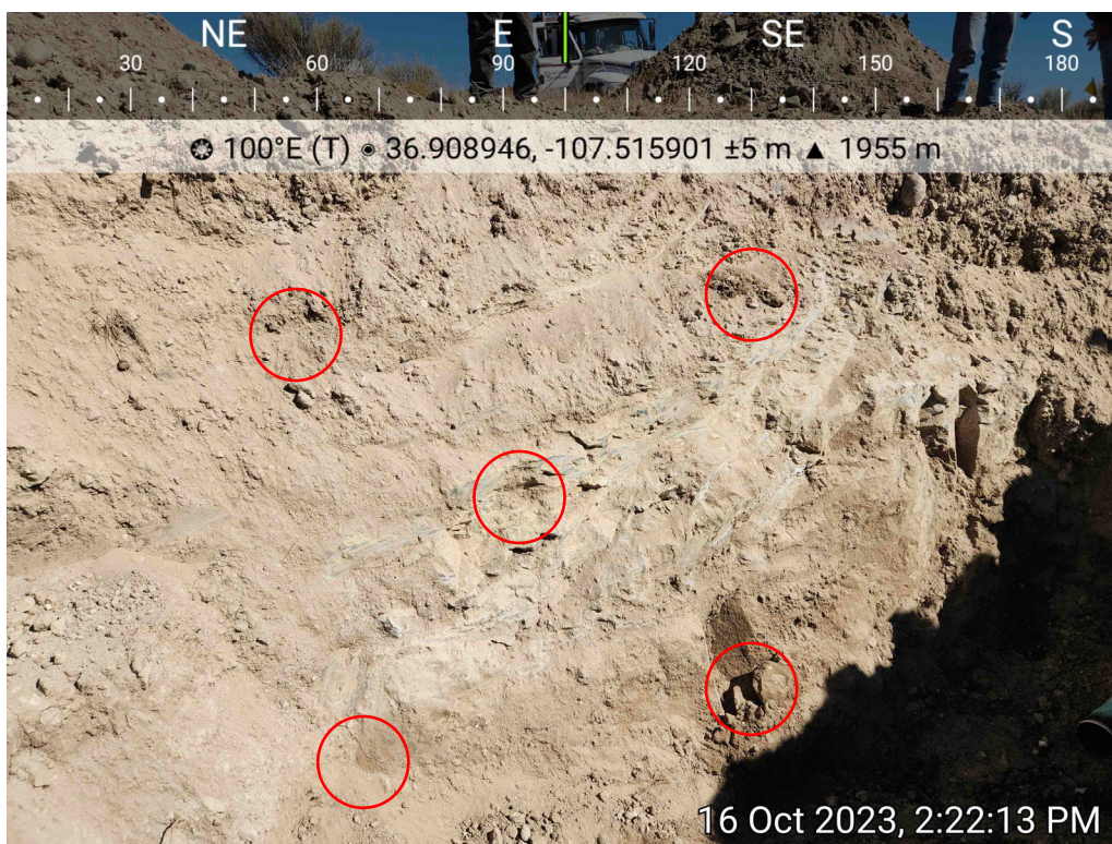
Photo 3: SS02 is a five-point composite sample collected from east sidewall, 10/16/2023.
