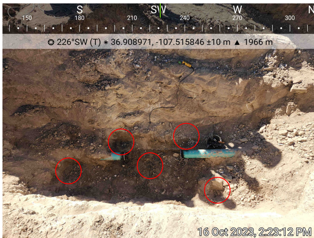
Photo 6: SS05 is a five-point composite sample collected from base of excavation, 10/16/2023.
