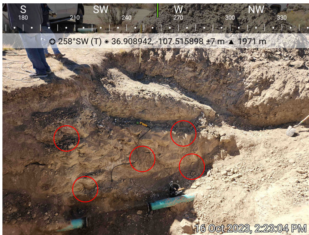
Photo 5: SS04 is a five-point composite sample collected from west sidewall, 10/16/2023.
