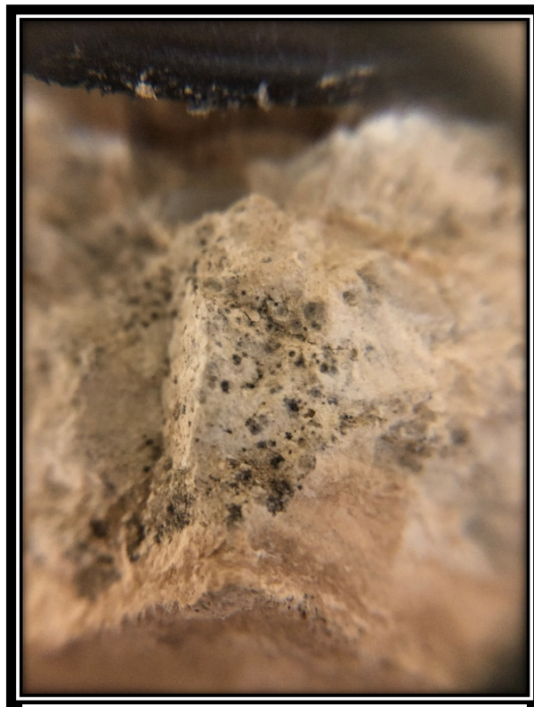
Photo 6: Crude Oil Trapped in Limestone at 20 feet in SB-8
