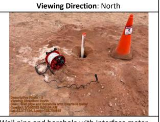
Well pipe and borehole with Interface meter
