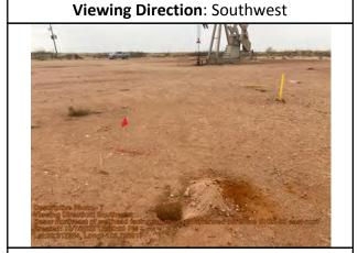
Northeast of wellhead facing southwest. Advanced borehole BH22-33 east-northeast of BH22-32 for horizontal delineation.
